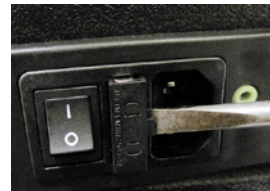
Picture 3: Unhinge the fuse cartridge with a flathead screwdriver
