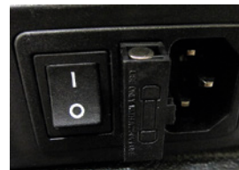
Picture 4: Replace the fuse and push the fuse cartridge back in place
