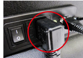
Picture 1: Remove the power cord
