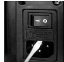
Picture 4: Unhinge the fuse cartridge with a flathead screwdriver.
